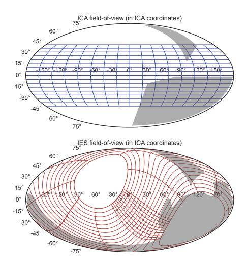
Figure S4. ICA (top panel) and IES (bottom panel) field-of-view, rotated into ICA instrument coordinates. The grid lines indicate the individual instrument pixels. The grey areas show obstructions in the field-of-view of the respective instrument due to spacecraft blockage.
