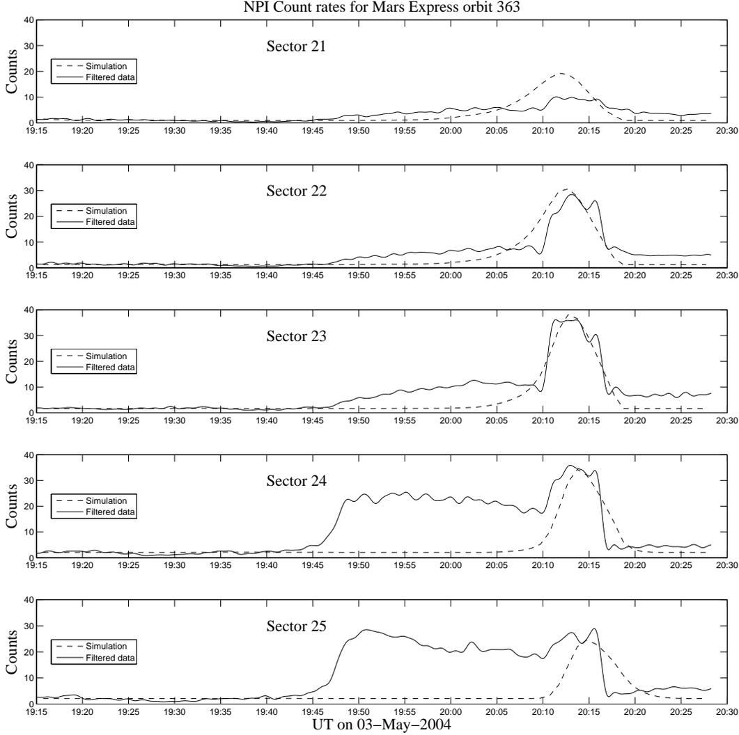
FIG. 4 Simulations (dashed curves) and filtered data (solid curves) from MEX orbit 363 and the ASPERA-3 NPI sensor. The highest count rates in sector 23 and 24 correspond to fluxes of  $1.3 \times 10^{11} \text{m}^{-2} \text{sr}^{-1} \text{s}^{-1}$  and  $1.2 \times 10^{11} \text{m}^{-2} \text{sr}^{-1} \text{s}^{-1}$  respectively. The dark counts shown in Table II have been added to the simulation results.
