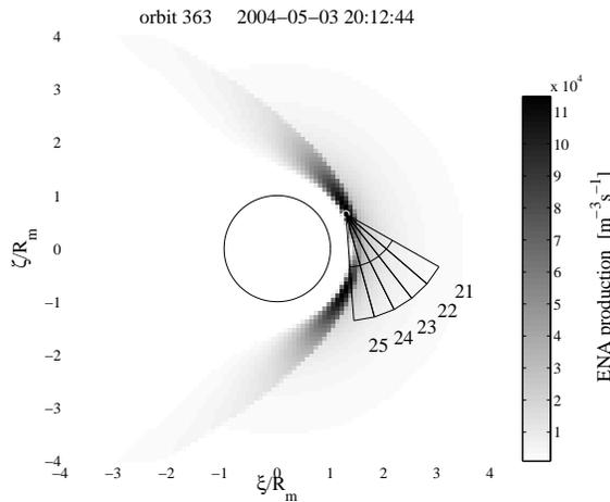
FIG. 2 Spacecraft position and field of view of sectors 21–25 at 20:12:44 UT on 3 May 2004. The grey-scale map shows a simulation of the ENA production rate in a plane that intersects the centre of all NPI sectors. The  $\xi$ -axis is the projection of the Mars-Sun line in the NPI plane, and the  $\zeta$ -axis is perpendicular to both the  $\xi$ -axis and the Mars-Sun line.
