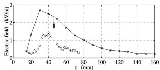
FIG. 3. The maximum electric field amplitude as a function of the axial coordinate  $z$  (solid curve). Also shown are the results of simultaneous three probe measurements. Measurements made with probe A, which is closest to the cathode, are marked “ $\times$ ,” probe B “+,” and probe C “ $\circ$ .” There is clearly an HF spike, as in the double layer case.
