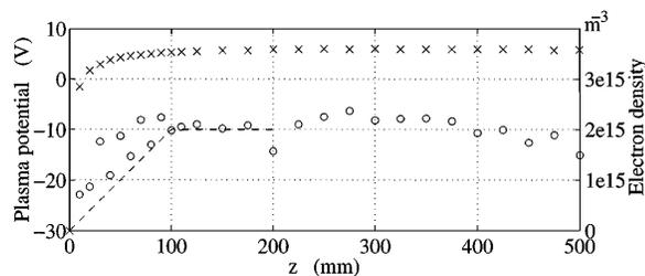
FIG. 2. Plasma potential ( $\times$ ) and density ( $\circ$ ) measured along the axis of the experimental device. The dashed curve shows the initial plasma density profile in the simulation.
