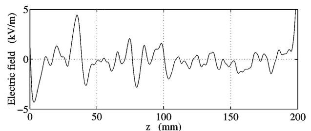
FIG. 6. The simulated electric field at time  $t = 3.00289 \mu\text{s}$ . The field spike is at about  $z = 35$  mm. The position remains stationary, and the field oscillates between about  $\pm 4 \text{ kV/m}$ .
