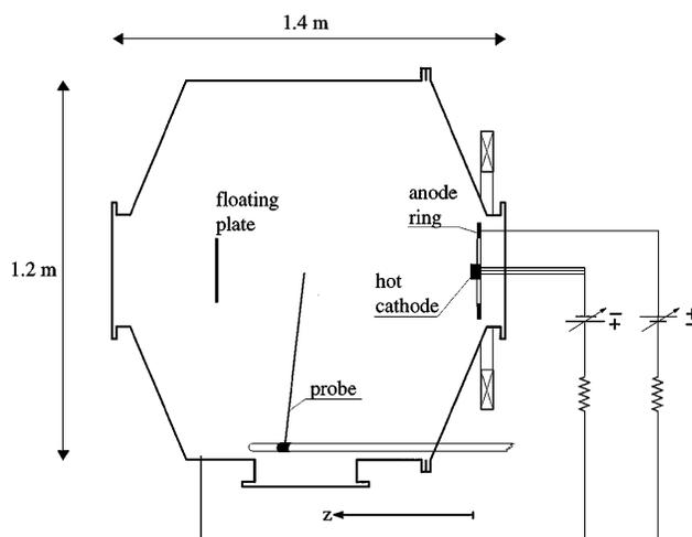
FIG. 1. The Green tank in which the experiments were performed. The electrons are accelerated in the cathode sheath and travel to the left in the figure.
