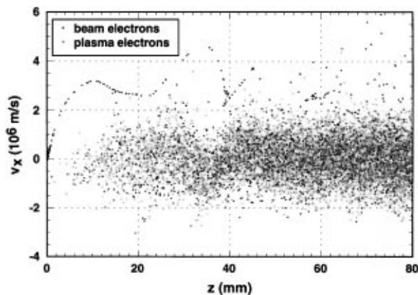
FIG. 7. Velocity phase space for beam and plasma electrons at time  $t = 3.00289 \mu\text{s}$ . The plot displays 80 mm of the 200 mm diode to emphasize the HF region. The position of the HF spike is about  $z = 35$  mm, and the beam is strongly dispersed after passing the spike.
