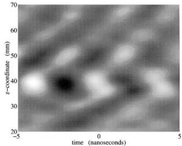
FIG. 5. The electric field of the wave as a function of time and space in the simulation. The similarity with the experimental data shown in Fig. 4 is conspicuous. Also in the simulation the total wave can be considered as a superposition of a traveling and a standing wave.
